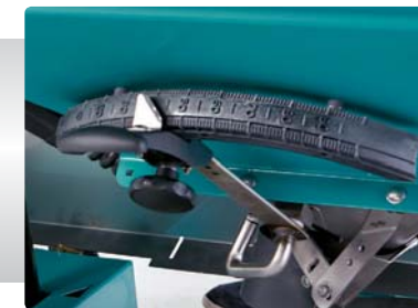
New easy-to-read graduated sectors for an application rate to the nearest kg
