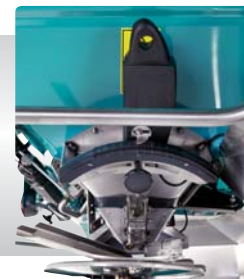
TRIBORD 2D: border device controlled from the cab
