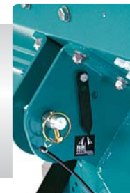
Level and angle indicator for late spreading
