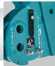
Level and angle indicator for late spreading
