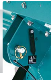
Level and angle indicator for late spreading
